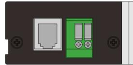
RJ11 or Terminal Block: Output door connection to indoor or inside cabinet
