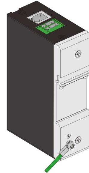
For DIN rail installation, the ground is via the DIN rail rack.
