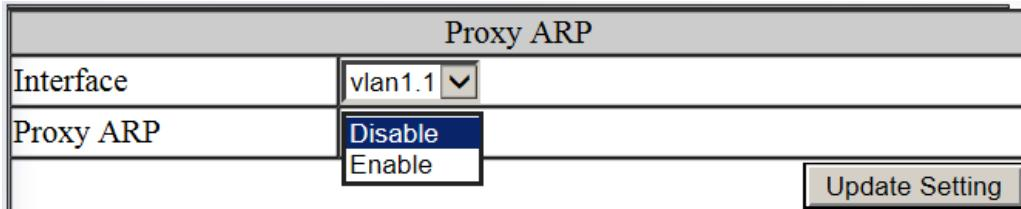
**Figure 114: Enable Proxy ARP on an interface**
