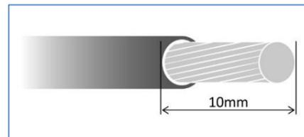
The power cord shall be IEC 60227 certified, rated 0.75 mm<sup>2</sup> x 3C or UL recognized minimum 18AWG.
