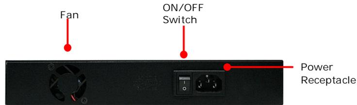
**Figure 2-2. Rear Panel of the EX17908 Switch**
