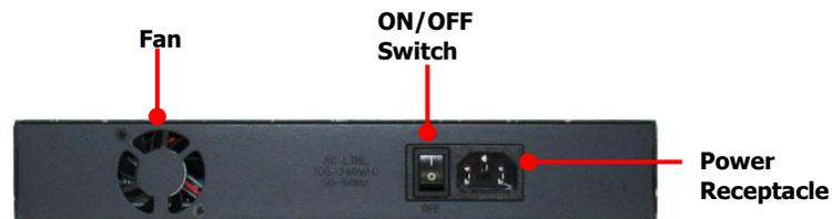
Figure 2-3. Rear Panel of the EX17008 Switch
