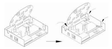
Bend the board of cable outlet hole.
