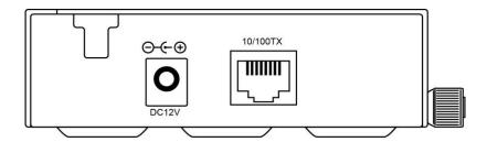
This 10/100BASE-TX to 100BASE-FX Media Converter is a plug-and-play device. Connect the supplied AC to DC power adaptor to the receptacle on the front panel of the 10/100BASE-TX to 100BASE-FX Media Converter, and then attach the plug into a standard AC outlet.
