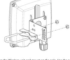
Position the Wireless unit and mount on the pole. Use the supplied U-Bolt and position the Wireless unit as shown in the graphic below. Once the wireless unit is in position, tighten the supplied nuts with washers to the U-Bolt until the Wireless unit is securely attached to the pole.
