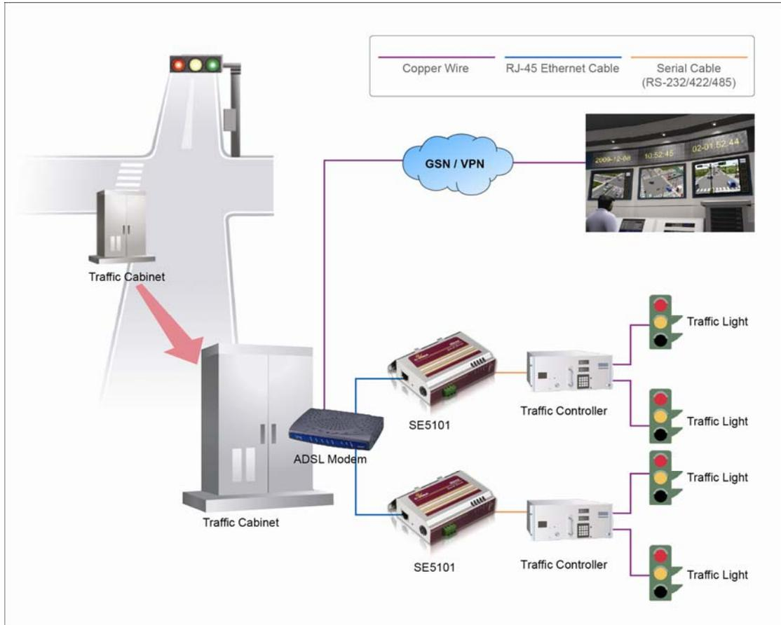
The controllers at the traffic control center can receive the signals from each intersection and respond through real-time control by sharing information. Owing to its wide operating temperature range, from -10°C to 60°C, and compact mechanical design, SE5101 is heat-resistant and flexible. Thus, it can be installed in a small cabinet under a harsh environment.
